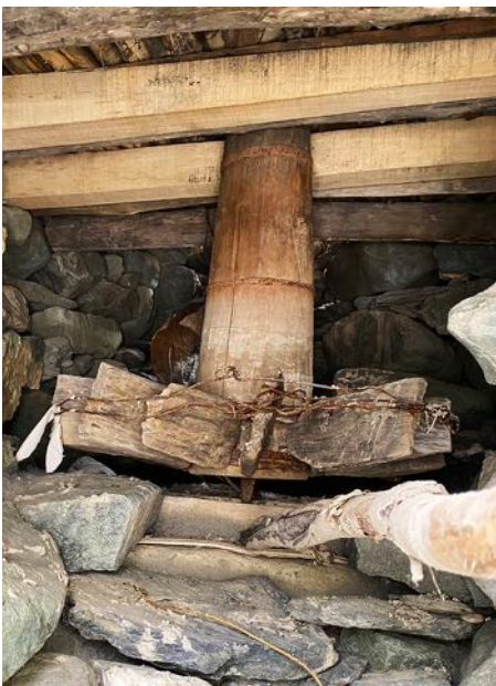
Figure 25 The various working components of the ranthak. Wooden turbine
